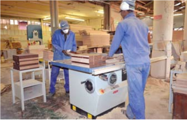
Operators using the rip saw which was supplied by Donald Fuchs Machinery
